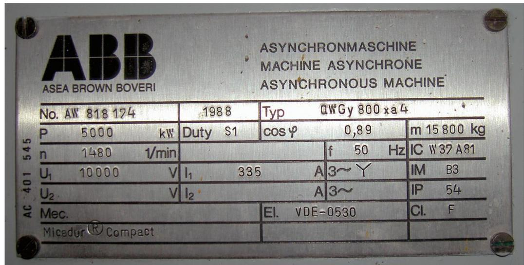
The image shows a metal nameplate for an ABB asynchronous motor. The plate is divided into several sections. At the top left is the ABB logo with 'ASEA BROWN BOVERI' underneath. To the right, the text 'ASYNCHRONMASCHINE', 'MACHINE ASYNCHRONÉ', and 'ASYNCHRONOUS MACHINE' is printed. Below this is a table of technical specifications. On the left side of the table, the vertical text 'AC 401 545' is visible. The table contains the following data:
